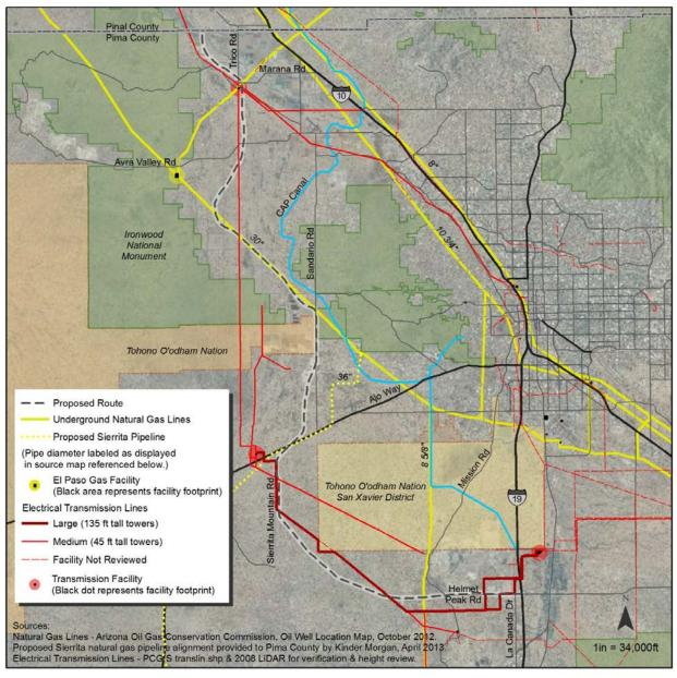
Figure 4: Natural Gas and Electrical Transmission Facilities
