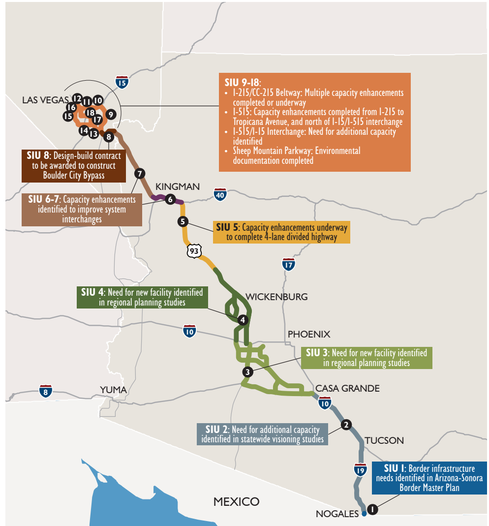
Figure 17 Illustrates the corridor’s 18 segments of independent utility (SIU), which are colored to clearly illustrate SIU endpoints. The status of project development activities completed to date are noted for each SIU. This segmentation does not include the Northern Nevada Future Connectivity Corridor segment, which requires additional study to determine logical corridor connections.
