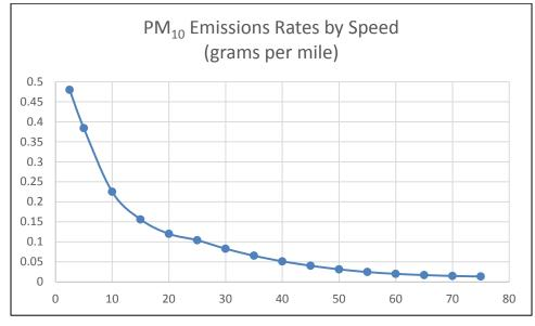
Figure 3.10-9 FHWA PM<sub>10</sub> Emissions Factors by Speed for Light-Duty Vehicles and Trucks, 2018
